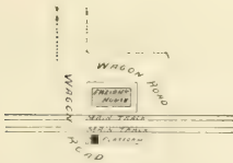
FIG. 351.—GENERAL LAYOUT AT LOCAL FREIGHT-STATION WITHOUT SIDINGS.
