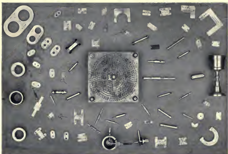
GAUGES MADE AT CREWE AND USED FOR THE MANUFACTURE OF GRAZE-FUSES.
