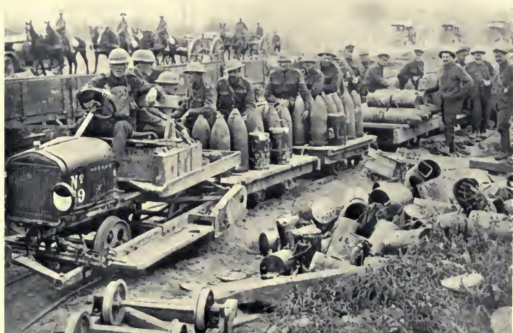
A CREWE TRACTOR AS LIGHT-RAILWAY ENGINE ON ACTIVE SERVICE.
