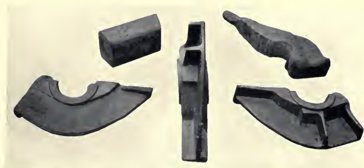
TRUNNION BRACKETS FOR 6-INCH HOWITZER GUN, DROP FORGING.
