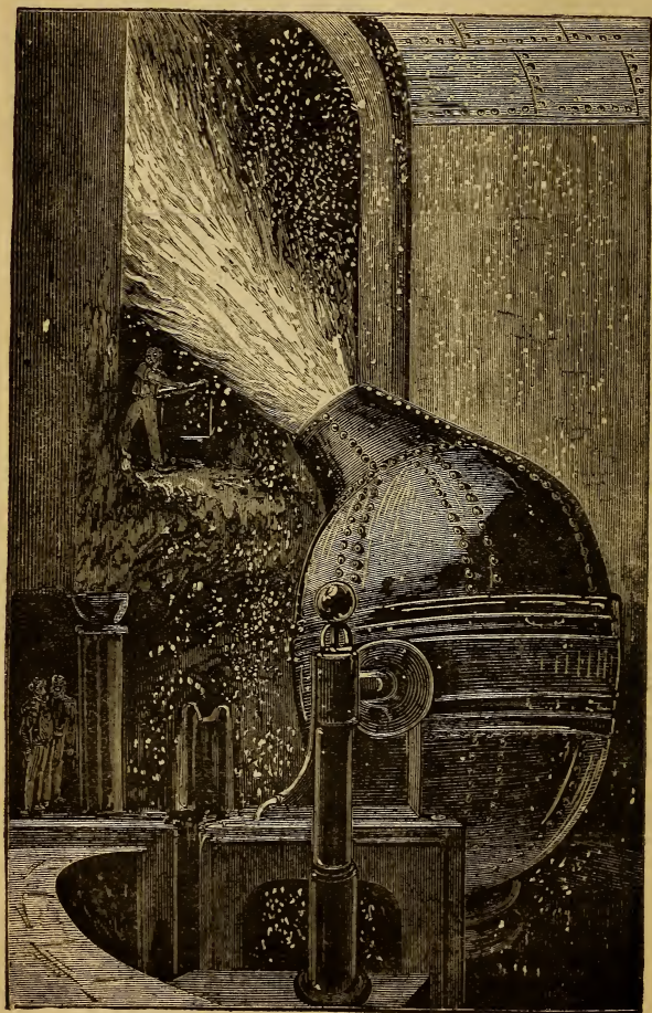
Retort for making Bessemer Steel. (Fig. 7.)
