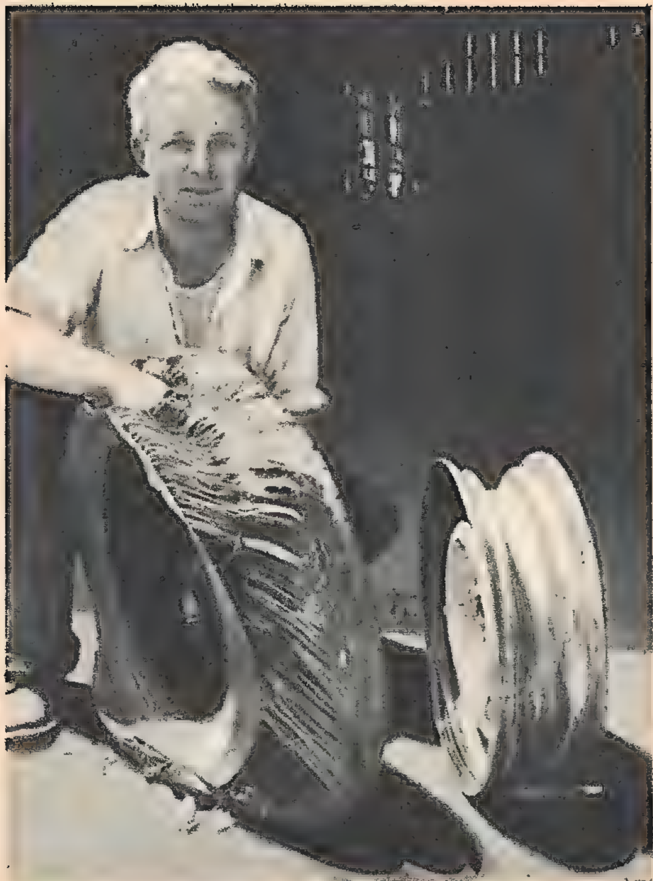
This automobile wheel, invented by Chris Sauer, of Chico, Calif., is said to eliminate blowout accidents by locking deflated tire to it, making the two one unit. Although torn to shreds, test tire remained locked to wheel at 65 m.p.h.
