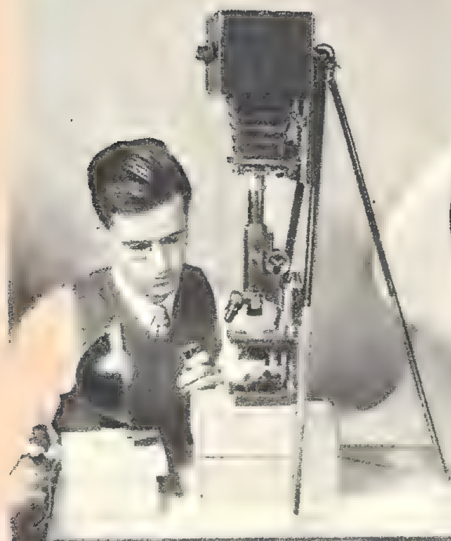
Many set-ups may be used in taking photomicrographs. Here a plate camera is supported over the microscope on a tripod, while blocks of wood elevate the microscope to correct height. Desk lamp light source appears at the extreme left.
