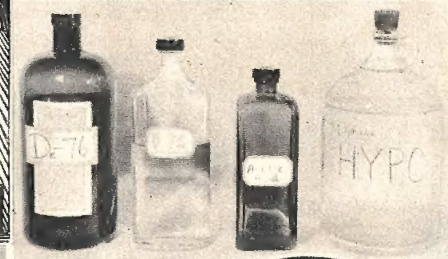
While chemical bottles of uniform shape and size look nice on the darkroom shelf, it is better practice to use containers that are physically different so that their contents can be instantly recognized when working in darkness. Bottles suitable for developing and fixing solutions are shown in photograph at left.
