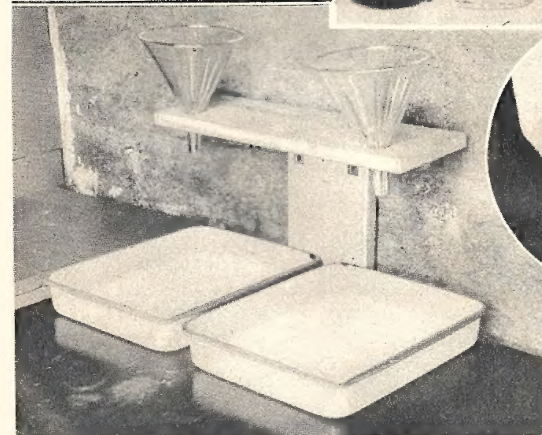
A permanent shelf for supporting 2 or 3 glass funnels is a great timesaver when both developer and hypo are to be filtered at the same time. Space holes so that 2 trays or tanks can be placed side by side. Shelf can be fastened to worktable with a short upright.
