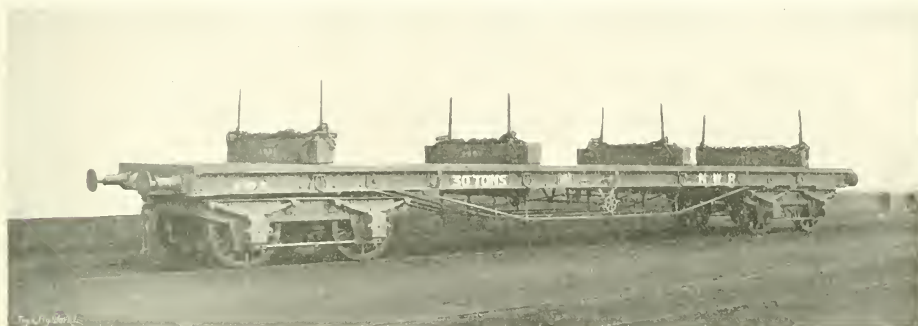
Thirty-Ton Platform Trolley with Bolsters (London and North Western Railway).
