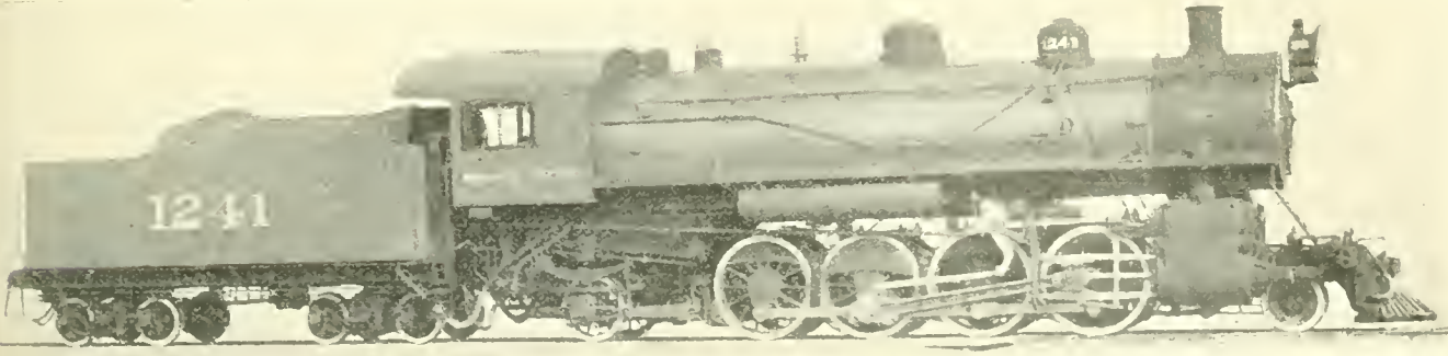
Goods Engine with Super Heater—Missouri Pacific Railway.
