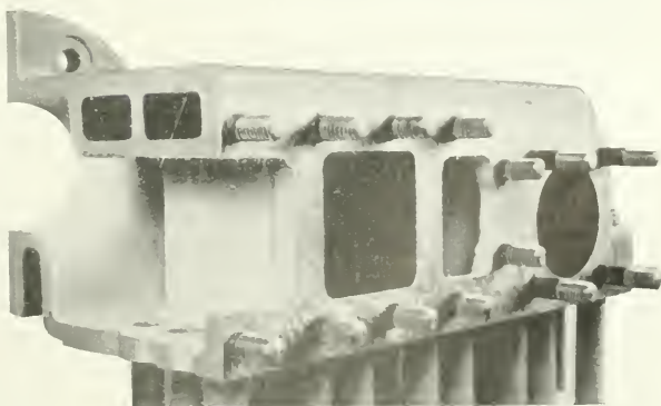
Half Sectional View of Header
