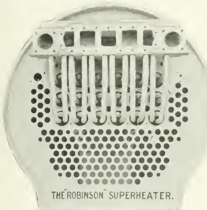
Front Cover Plate Removed.
