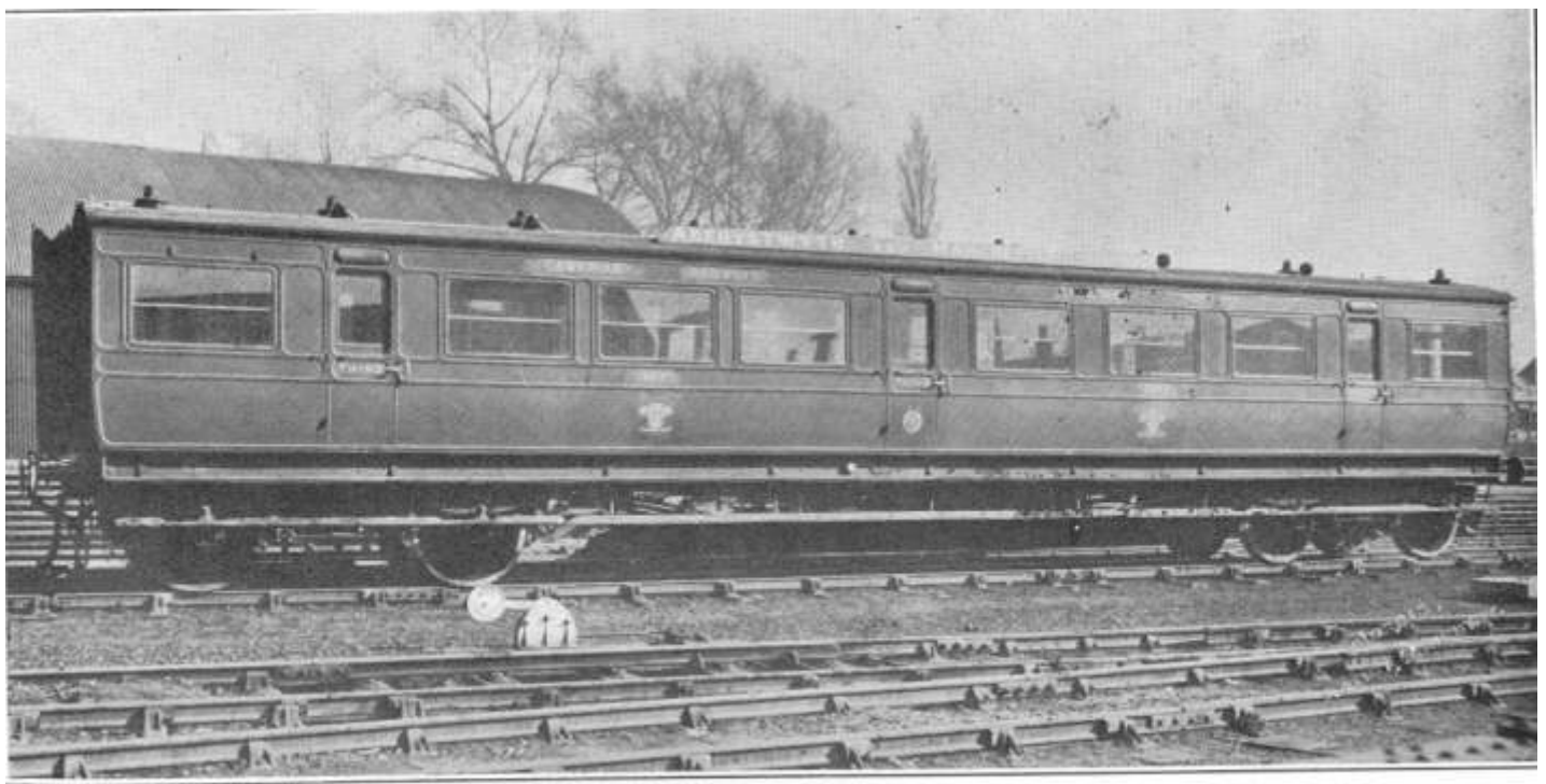
Latest Cambrian Composite Bogey Coach, built for through traffic between Aberystwyth and Manchester.
