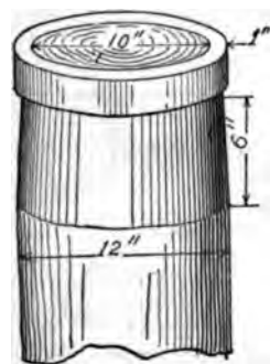
FIG. 18.—RING FOR PILE.
